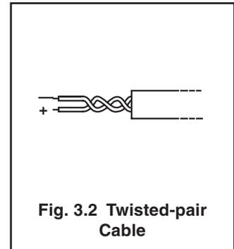
Shielded twisted-pair wire, which will reduce the effects of electromagnetic and electrostatic noise coupling, should be used for analog signal connections, as shown in Figure 3.2.
