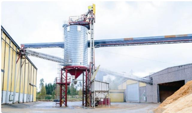
Build-up on vessel walls and constant profile changes are real challenges for most non-contact level measurement technologies. These changes in the vessel change the way beams emitted by the instruments are detected. This often requires another mapping of the vessel, which is time consuming and costly.
