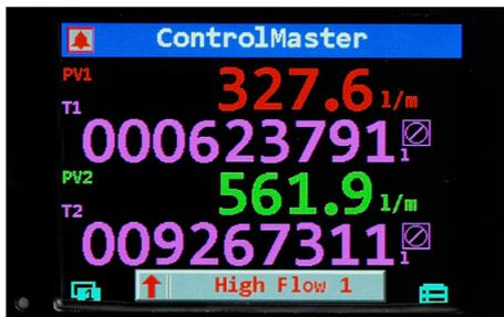
Figure 3 Dual PV and totalization display
