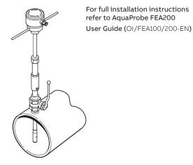
Figure 6 Typical installation (metal pipe)
