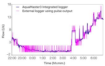
Figure 4 Elimination of pulse quantization with AquaMaster3
