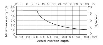
Figure 7 Maximum allowable velocity for different insertion lengths
