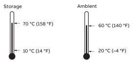
Operation outside ambient temperature limits of 0 to 45 °C (32 to 113 °F) reduces battery capacity and shortens battery life.
