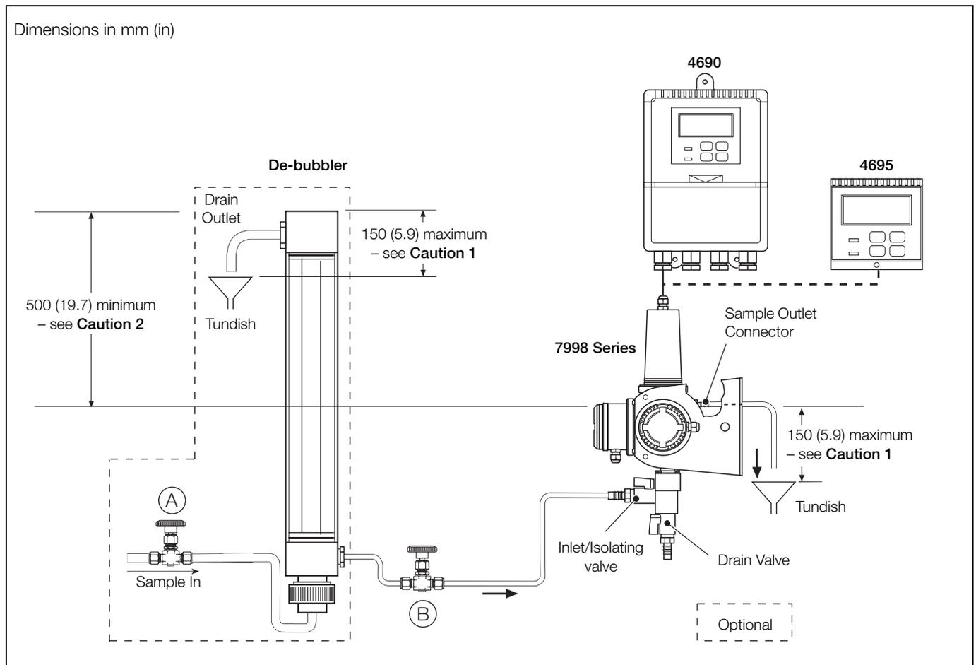
Fig. 3.12 Typical System Installation for 7998 Series Turbidity Systems
