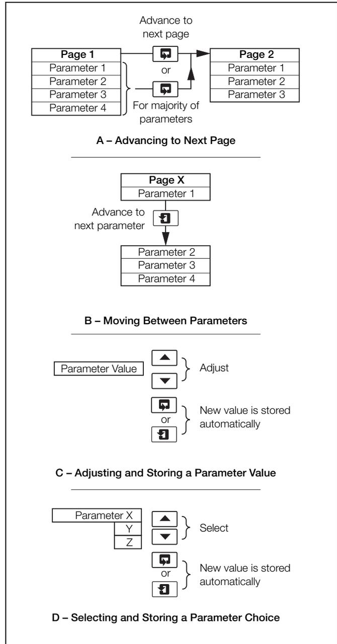
Fig. 5.2 Membrane Key Functions
