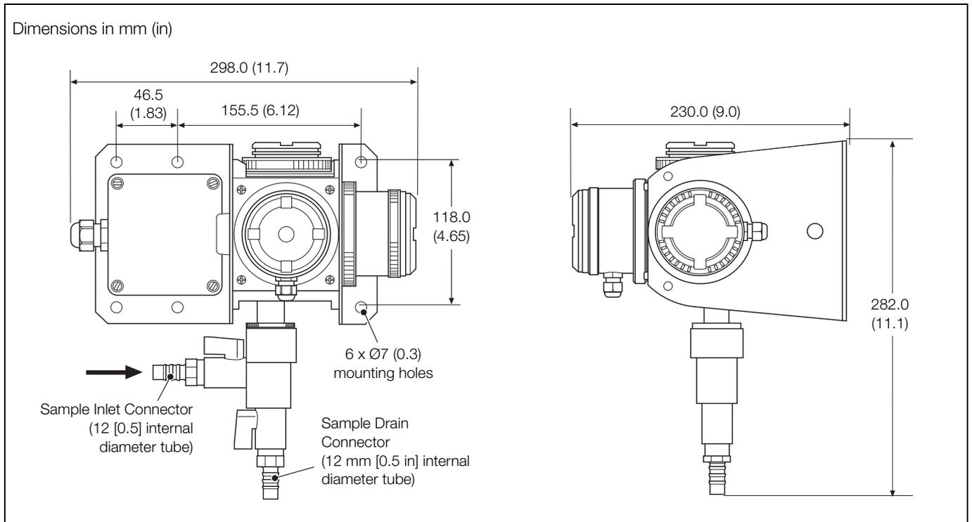
Fig. 3.9 Sensor Dimensions (Without Optional Wiper Unit)
