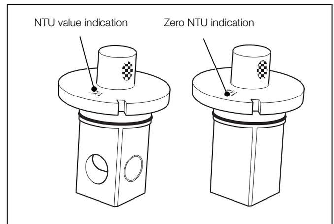
Fig. 7.3 Dry Calibration Standard for High Range Sensors
