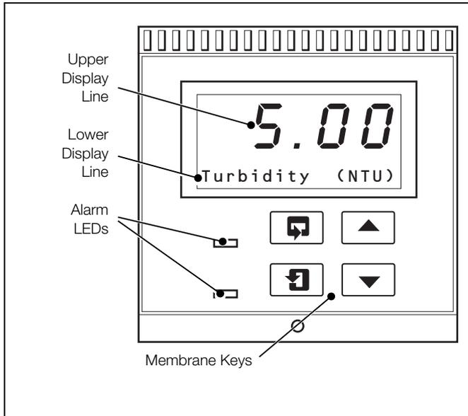
Fig. 5.1 Controls and Display
