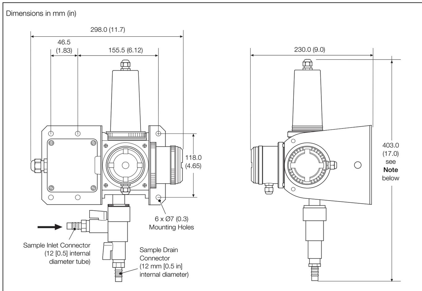
Fig. 3.8 Sensor Dimensions (With Optional Wiper Unit)
