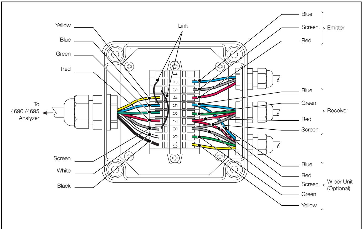
Fig. 4.9 Turbidity Sensor Junction Box Connections
