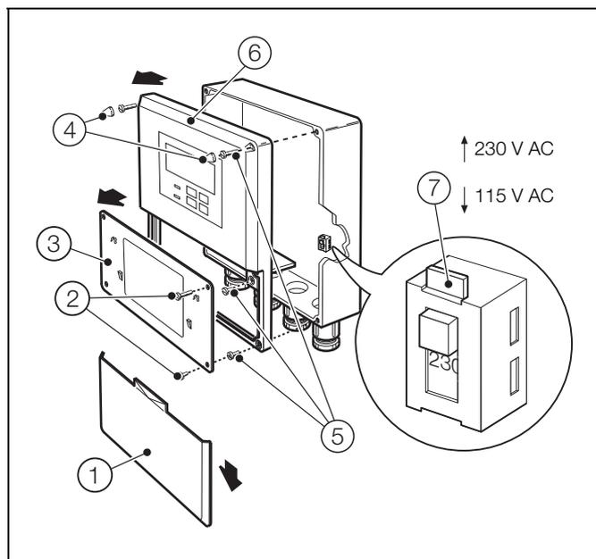
Fig. 4.7 Selecting Mains Voltage – Wall- / Pipe-mount Analyzer
