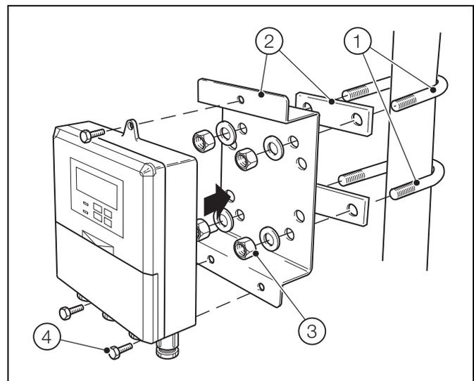
Fig. 3.5 Pipe-mounting
