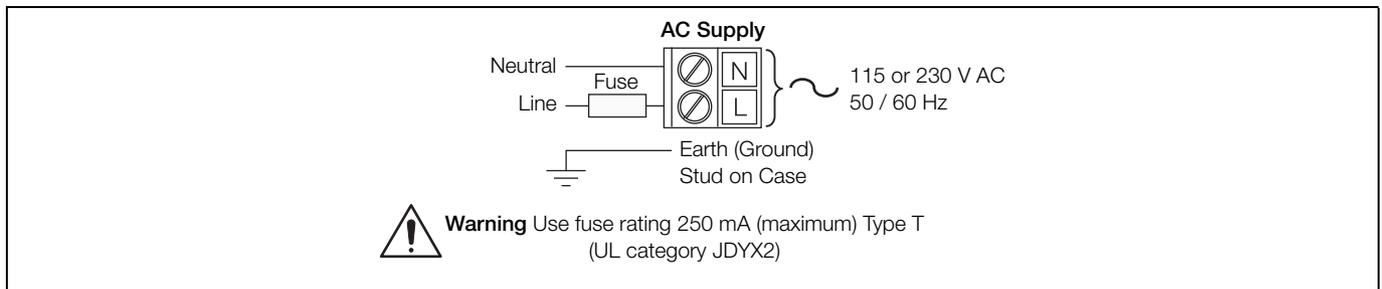
Fig. 4.6 AC Power Supply Connections
