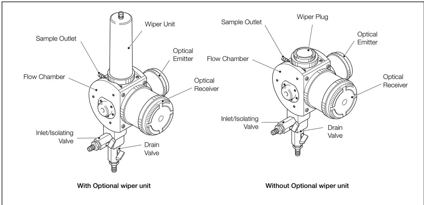
Fig. 2.2 Turbidity Sensors – Main Components
