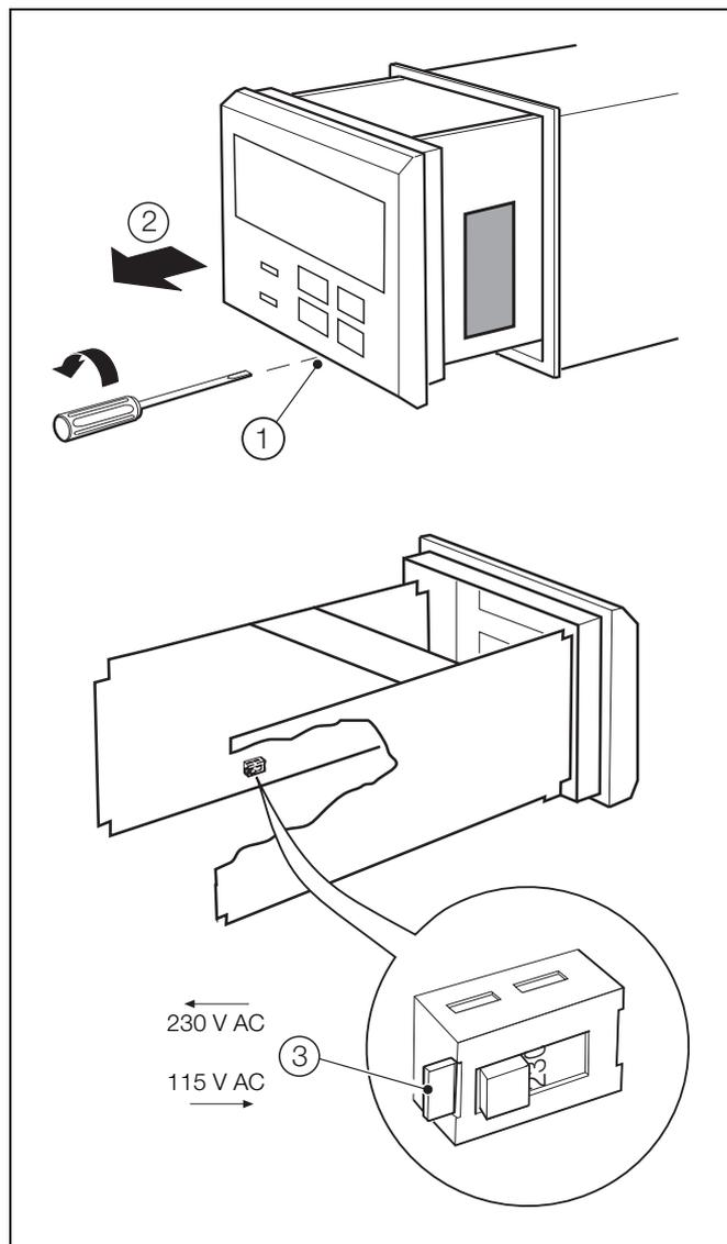
Fig. 4.8 Selecting Mains Voltage – Panel-mount Analyzer
