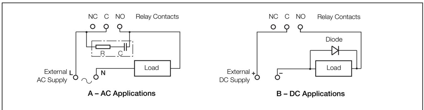
Fig. 4.3 Relay Contact Protection
