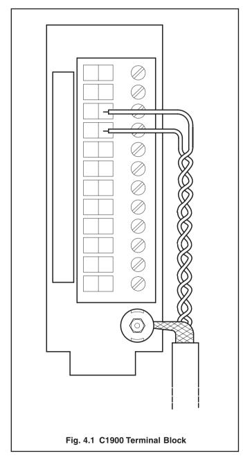
If a double-shielded wire is used, ground the inner shield at one end and ground the outer shield at the other end.
