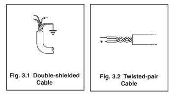
Shielded twisted-pair wire, which will reduce the effects of electromagnetic and electrostatic noise coupling, should be used for analog signal connections, as shown in Figure 3.2.
