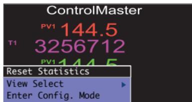
Operator level menus are used to reset statistics, select the view and to enter *Basic* and *Advanced* modes (via the *Access Level*).
