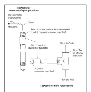
Typical Threaded Sensor Installation – TB(X)556 pH Sensor
