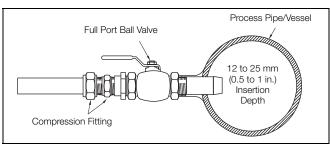
Typical Retractable Sensor Installation – TB(X)587, TB(X)557 or TB(X)564 pH Sensor
