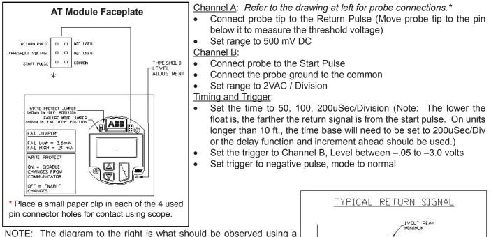
NOTE: The diagram to the right is what should be observed using a dual channel oscilloscope. If the float were upside down, the Return Pulse would be inverted. If noise is present, it would show up on the baseline.
