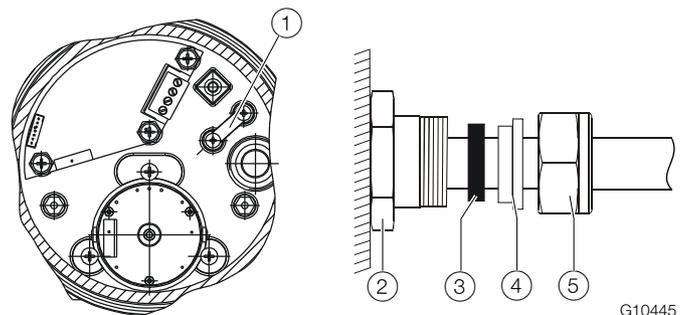
**Fig. 5: Connection using a flameproof cable gland**
