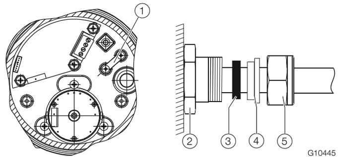
**Fig. 1: Connection using a flameproof cable gland**
