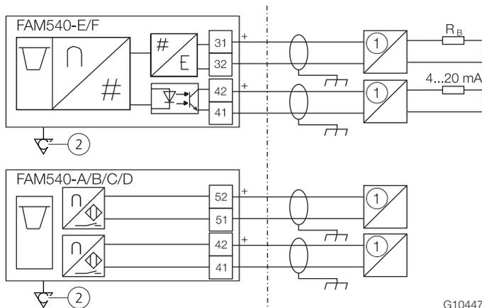
**Fig. 6: FM / cCSAus electrical connection**
