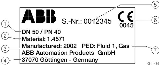
Fig. 11: Factory plate for meter tube size  $> DN 25$  (example)
