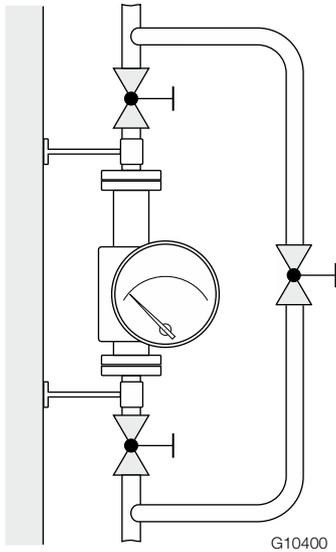
Fig. 13: Installation of the flowmeter (example)
