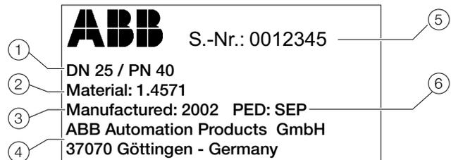
Fig. 12: Factory plate for meter tube size  $\leq DN 25$  (example)
