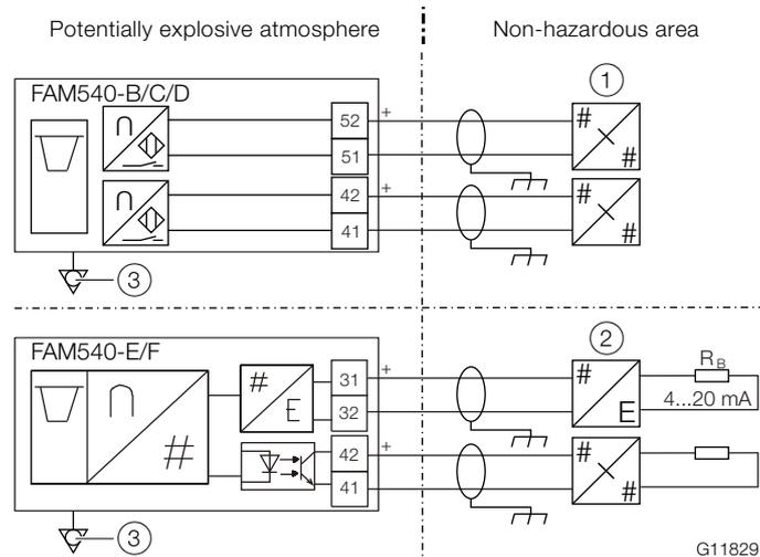
**Fig. 2: ATEX / IECEx electrical connection**
