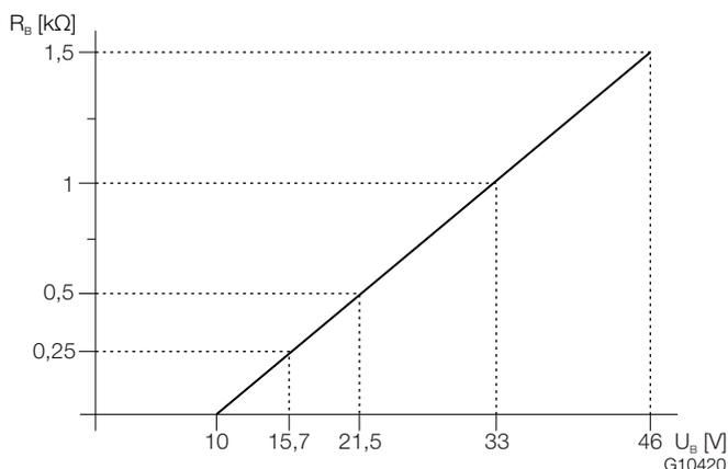
Fig. 25: Load diagram of the current output
