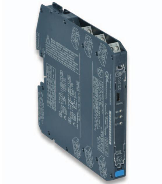
D5072S-089, D5072D-089, are Universal Converters and share the same screens, except for the number of input and output channels. Voltage Output.
