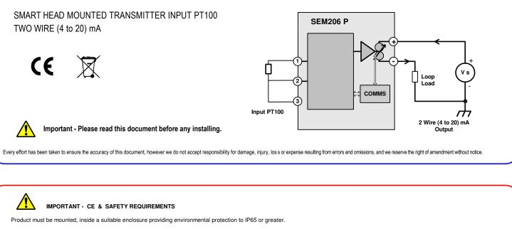
To maintain CE EMC requirements, input wires must be less than 3 metres.
