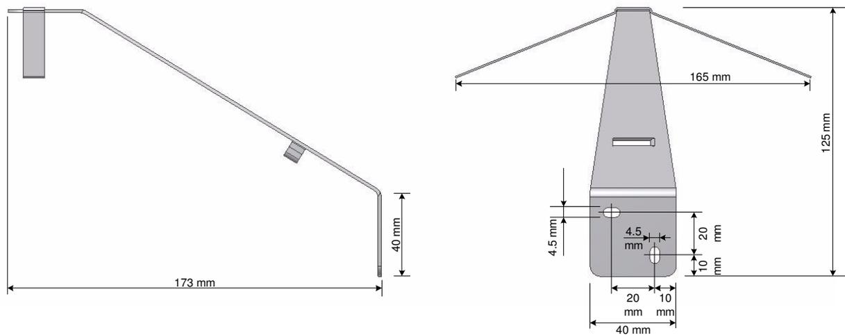
Figure 10: Dimensions of antenna wall holder for lambda/4 antenna
