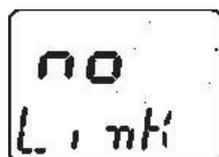
Figure 20: Display when no linked channels are available
