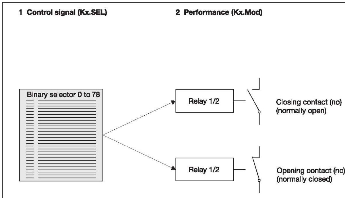
Figure 2: Performance of the relay outputs 1 to 2
