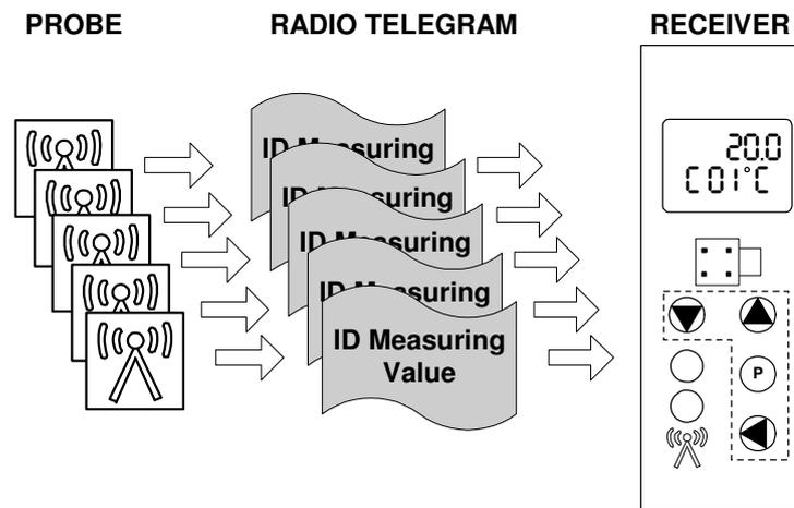
Figure 4: Telegrams of several probes can collide.
