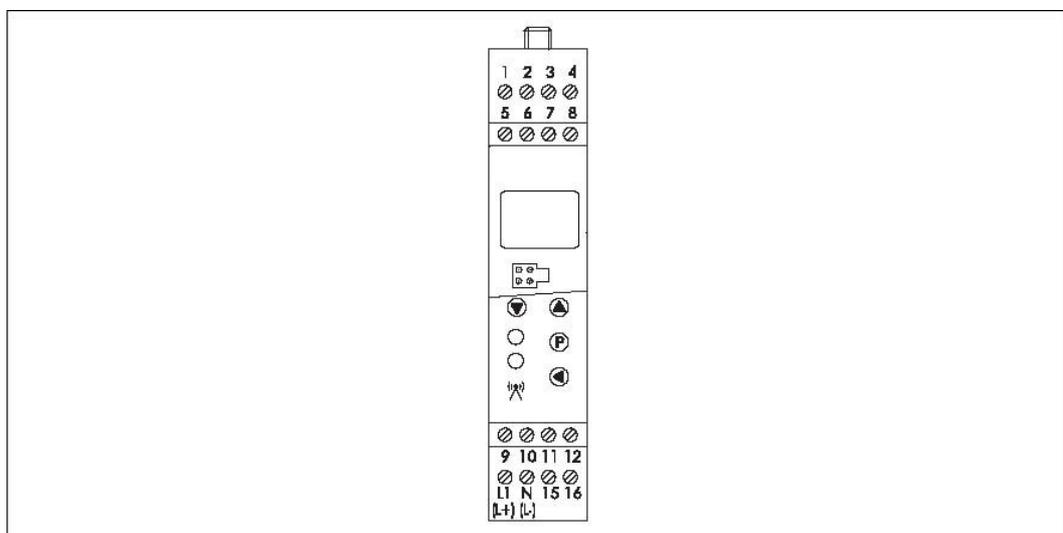
Figure 14: Front view with terminal designation
