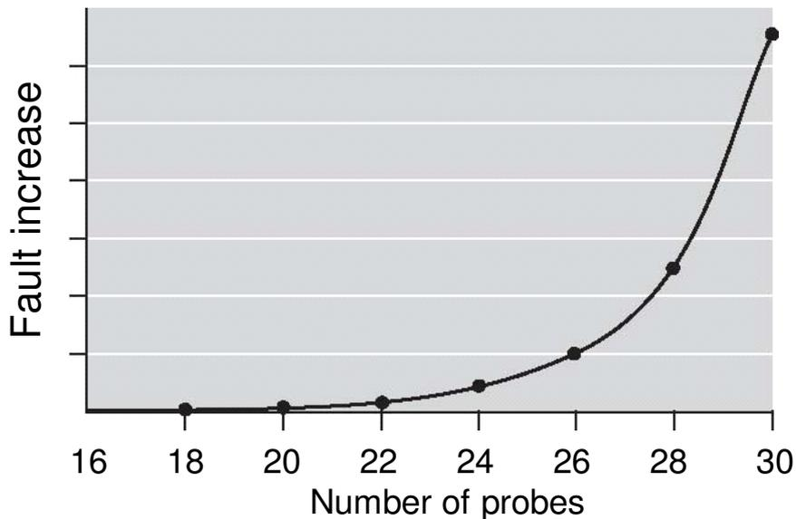
Figure 5: Collisions depending on the number of probes at a transmission interval of 1 s
