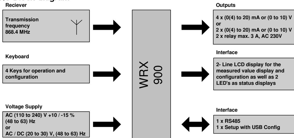
Figure 1: Receiver block diagram
