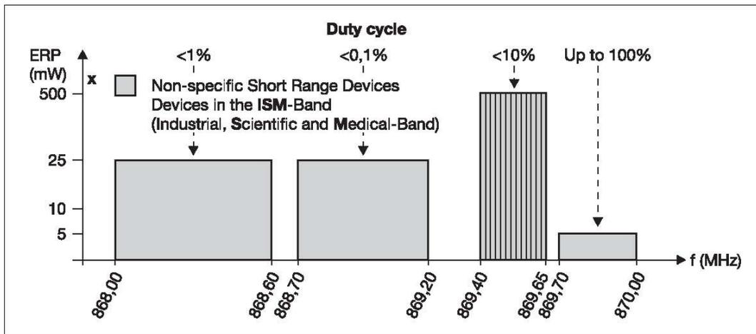
Figure 1: Subdivision of the 868 MHz frequency band
