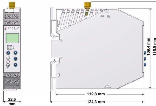
Figure 8: Receiver dimensions
