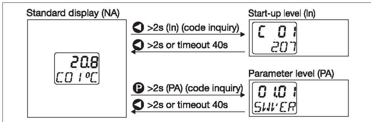
Figure 22: Change-over to different levels
