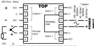
USE COPPER CONDUCTORS (EXCEPT FOR TC INPUT)
