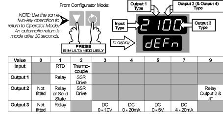
\* Dual Relay Option PCB must be fitted.
