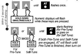
NOTE: Pre-Tune will not engage (a) if the setpoint is ramping, (b) if the process variable is within 5% of input span of the setpoint, (c) if the proportional band = 0 or (d) if Soft Start is operating. It is a single-shot routine and is thus self-disengaging. If **FPE** = 1 (Auto Pre-Tune enabled - see SET UP MODE), Pre-Tune will run for every power-up.
