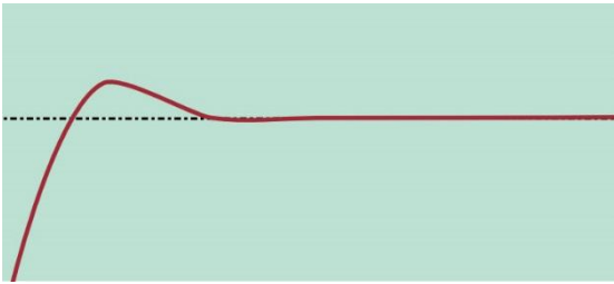
Too Small: Overshoots setpoint before settling
